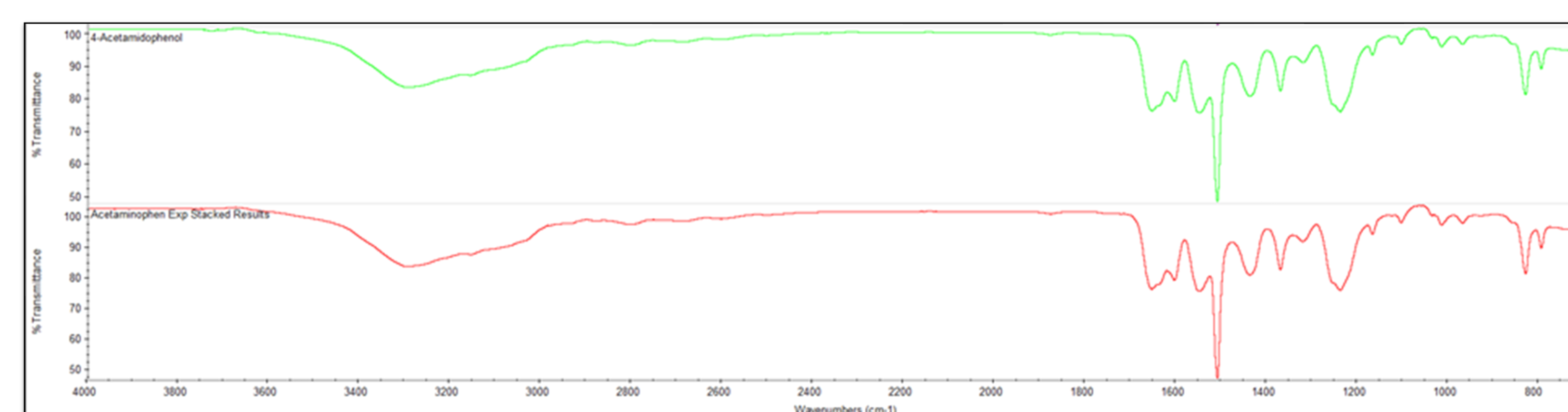
Figure 2. Expected IR on top in green from reference acetaminophen (Acros Organics, Product #102330050, CAS No: 103-90-2) and Experimental IR on bottom in Red from recrystallized product
